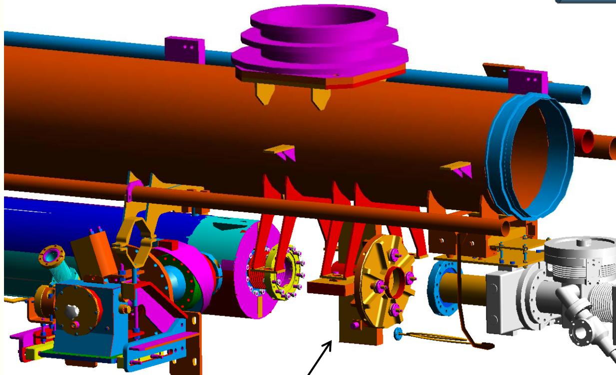
ILC type cold CM-free L-Band cavity BPM
