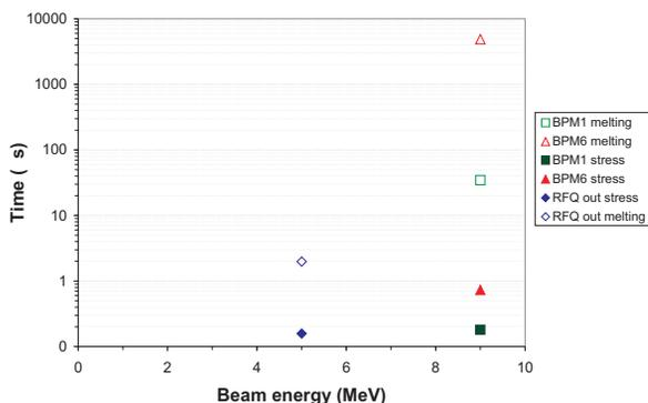
Figure 4: Damage time caused by an out-of-control bunch impacting perpendicularly to a stainless steel wall.
