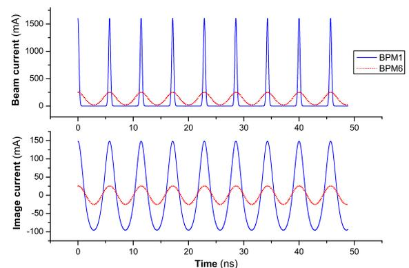
Figure 2: Comparison of the beam and image current at different BPM positions along the diagnostics plate.
