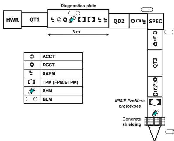
Figure 1: Sketch of the position of the main diagnostics along the HEBT. The lengths of the elements are approximative and scaled. Definition of the acronyms are given along the text.
