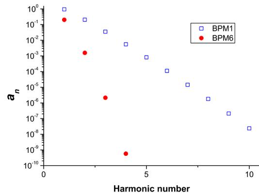
Figure 3: Comparison of the frequency components of the image current at the beginning (BPM1 position) and end (BPM6 position) of the HEBT.
