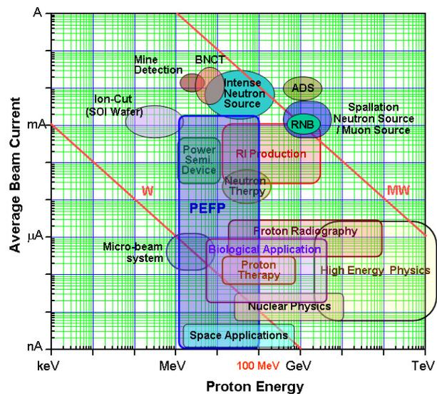
Figure 1: Utilization and application of proton beams depending on energy and current: the PEFP linac can cover the shaded (blue) region.
