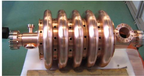
Figure 14: Copper model of PEFP low beta cavity.
