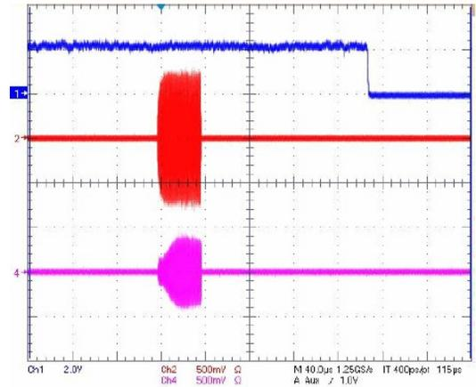
Figure 7: Beam current at the ends of the 3-MeV RFQ (middle, red) and the 20-MeV DTL (low, pink): peak beam current of 20.2 mA.
