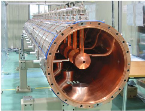
Figure 9: 100-MeV DTL tanks which is assembled at the KAERI site.
