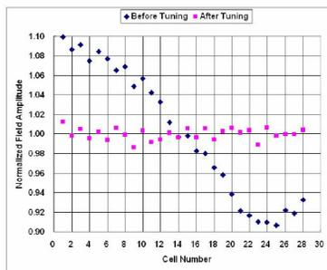
Figure 10: Normalized electric fields before and after tuning.
