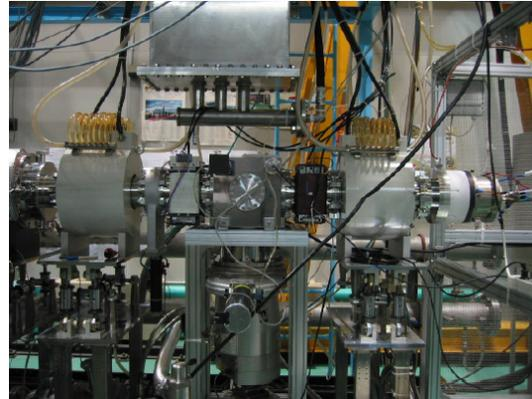
Figure 3: PEFP injector system including an ion source and a low energy beam transport.
