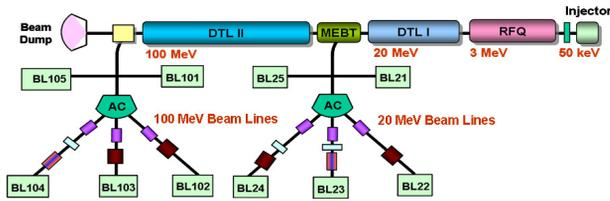
Figure 2: Schematic plot of the PEFP linac and beam lines.
