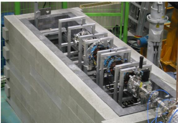
Figure 6: Target station for 20-MeV proton beam test.
