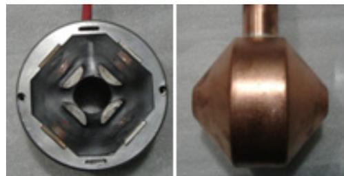
Figure 8: Quadrupole magnet and drift tube installed in the 100-MeV DTL tank.
