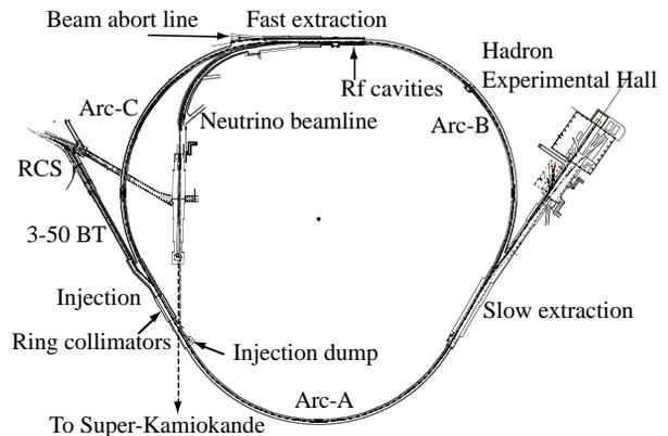
Figure 1: Layout of MR and experimental facilities.
