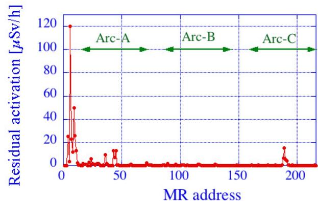
Figure 7: Residual activation after the first stage runs.
