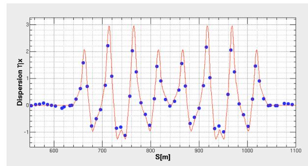
Figure 4: Horizontal dispersion function for one super-period. The solid line shows design and closed circles show measured results.
