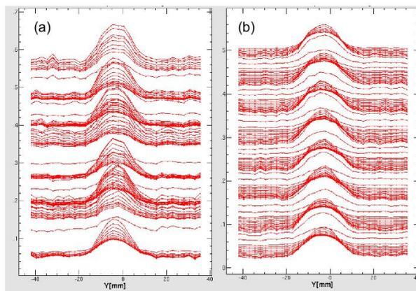
Figure 3: Mountain plots of vertical beam profile for (a) 16-23 turns and (b) 72-79 turns after the beam injection.
