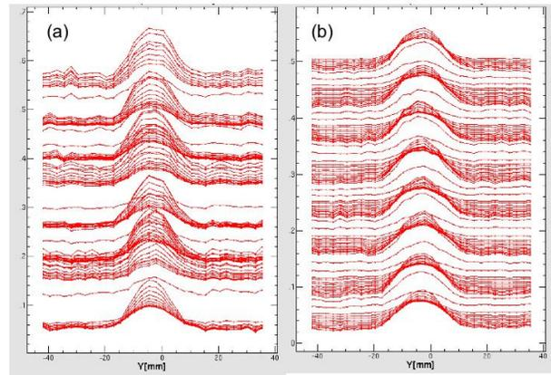
Figure 3: Mountain plots of vertical beam profile for (a) 16-23 turns and (b) 72-79 turns after the beam injection.
