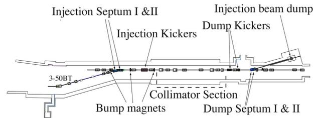
Figure 2: Injection and collimator section.
