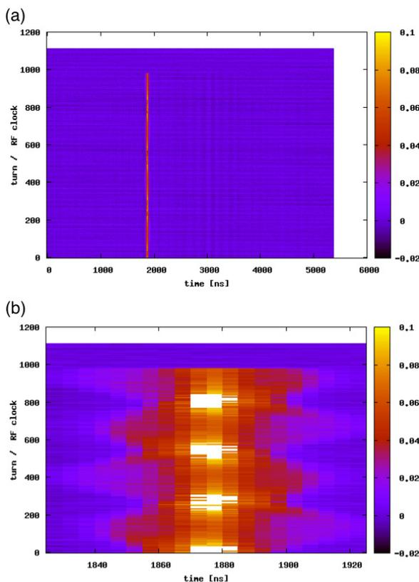
Figure 6: Mountain plots of longitudinal profile measured by the WCM. Time ranges are (a) 5.4 msec, (b) 100 nsec.
