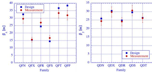
Figure 5: The beta function for each quadrupole family.
