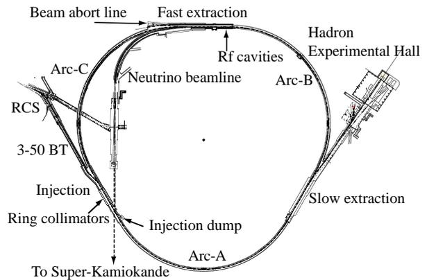
Figure 1: Layout of MR and experimental facilities.
