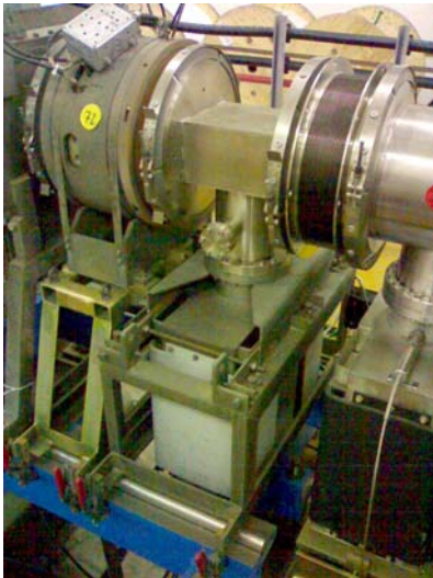
Figure 5: An ion pump assembly on the ISIS synchrotron showing various features outlined in the text to minimise radiation doses to maintenance workers.
