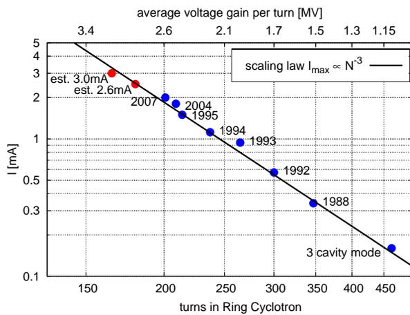
Figure 3: Development of the Ring Cyclotron beam intensity as a function of the turn number.
