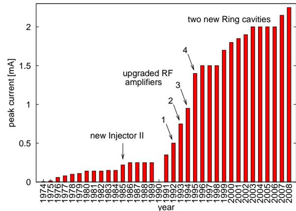
Figure 1: Development of the maximum accelerated beam current in the PSI proton accelerator over time.
