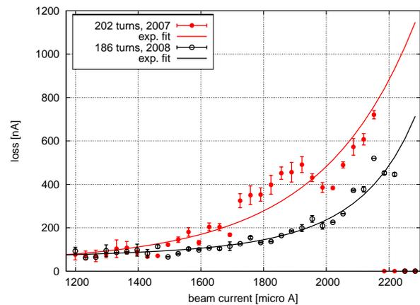
Figure 6: Loss current at the Ring Cyclotron extraction, deduced from ionization chamber rates, as function of beam current for the cases of 202 and 186 turns. The shown data points are taken at optimized situations, i.e. they represent the minimally achieved losses at each current.
