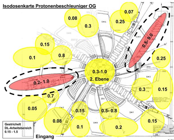
Figure 5: Results of dose rate measurements in mSv/h, in the Ring Cyclotron for a typical service situation (graphics provided by R. Küng, PSI).
