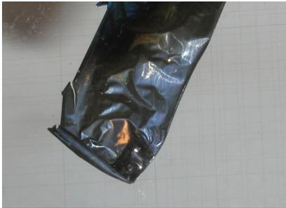
Figure 6: Curling, indicated by the strong change in the foil “thickness” variable (see figure 4), is evident in the DLC foil, which was removed from the ring after only two weeks of production beam exposure.
