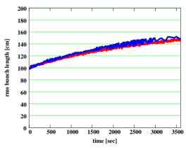
Figure 4: Time evolution of the RMS bunch length: blue curve – simulations, red curve – measurements.
