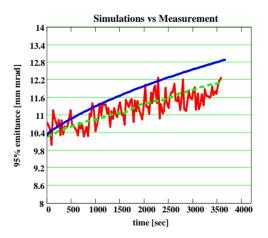
Figure 5: Time evolution of the 95% normalized horizontal emittance: red noisy curve – measurements; green dashed curve - simulations using  $95^{\circ}$  lattice; blue upper curve – simulations using  $82^{\circ}$  lattice.
