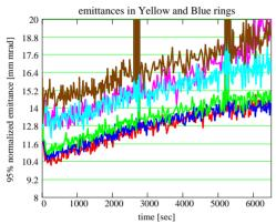
Figure 3: Horizontal emittances: 1) upper three curves – three high-intensity bunches in Blue ring; 2) lower three curves – three high-intensity bunches in Yellow ring.
