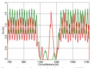
Figure 6: Design dispersion functions for two RHIC arcs for the 95° phase advance per FODO cell lattice (dAu82) and 82° lattice which were used in simulations for Fig. 5.
