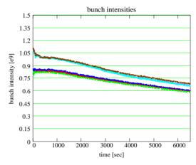
Figure 1: Bunch intensity: 1) upper three curves – three high-intensity bunches in the Blue ring; 2) lower three curves – three high-intensity bunches in the Yellow ring.
