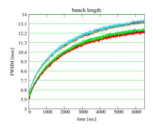
Figure 2: Bunch length: 1) upper three curves – three high-intensity bunches in the Blue ring; 2) lower three curves – three high-intensity bunches in the Yellow ring.
