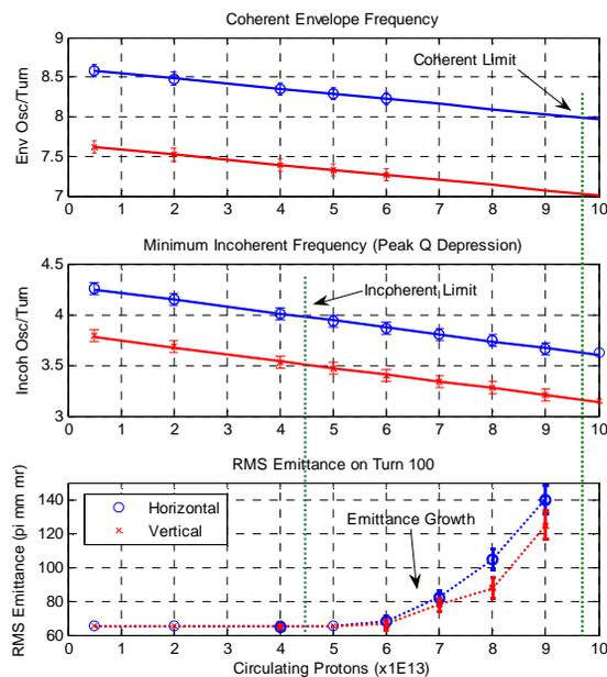
Figure 4: Intensity limits associated with half integer resonance and associated  $\epsilon_{RMS}$  growth.
