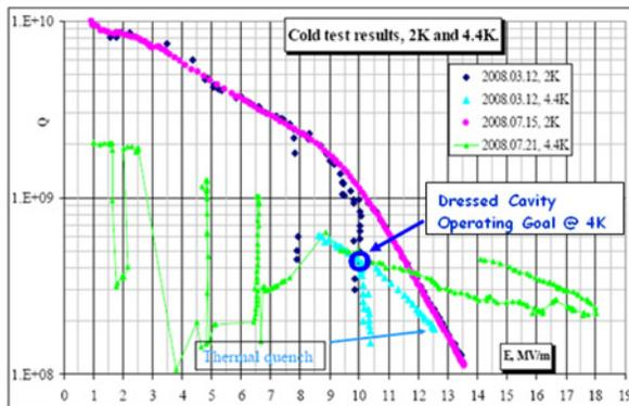
Figure 10: Q vs. Accelerating field plot for the first SSR1 prototype built for the HINS program. The operating goal is also indicated.
