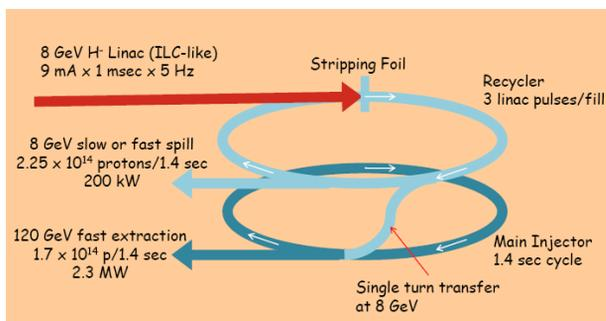
Figure 4: Project X schematic conception for an ILC-identical linac (9 mA x 1 msec x 5 Hz) injecting up to 3 pulses in the Recycler Ring.
