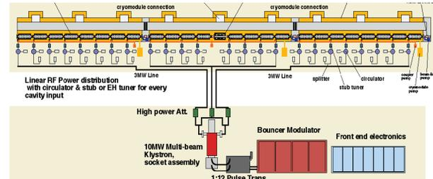
Figure 11: RF unit schematic.
