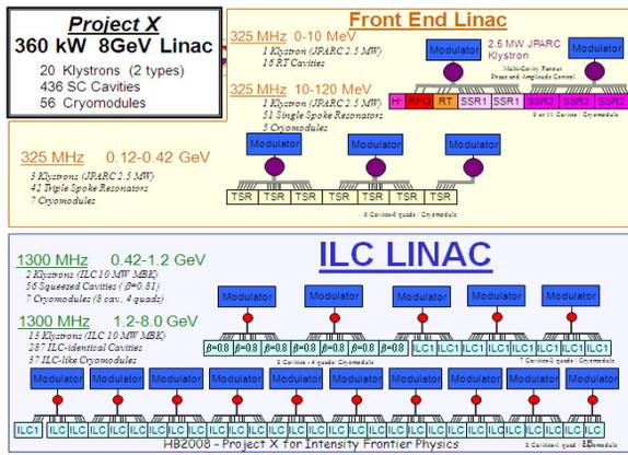
Figure 6: Schematic layout and components count for 8 GeV linac with ILC-identical components.
