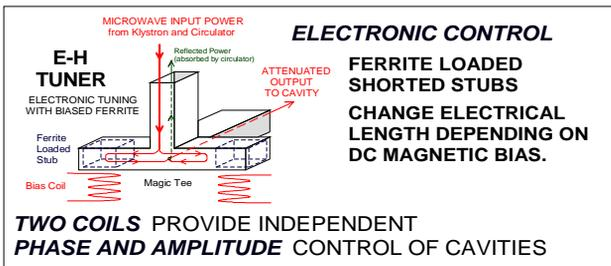
Figure 13: Conceptual principle of operation for a FVM controlling phase and amplitude of RF power
