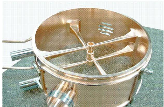
Figure 8: One normal-conducting resonator after brazing of the spokes and ready for welding of the flanges.
