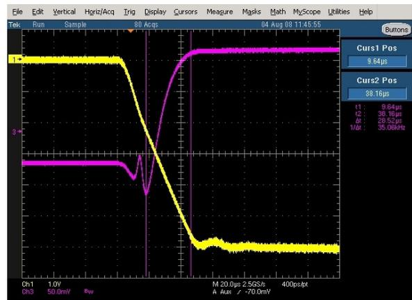
Figure 14b: 120 Degree Phase Control with Vector Modulator for a 300A current change in Vector Modulator coils bias current. The purple trace is the cavity RF phase signal (changing by 120° between the 2 vertical purple lines), the yellow trace is the bias currents.
