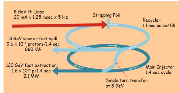
Figure 5: Project X schematic conception for a high-power linac (20 mA x 1.25 msec x 5 Hz) injecting 1 pulse in the Recycler Ring.
