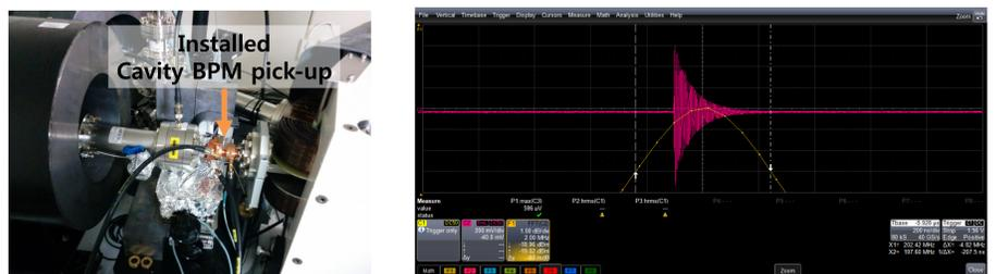
Figure 3. Installed Cavity BPM pick-up at ITF dump section and down converted raw signal of XY cavity y-direction port (200 MHz). Measured decaying time was  $\sim 30$  ns.
