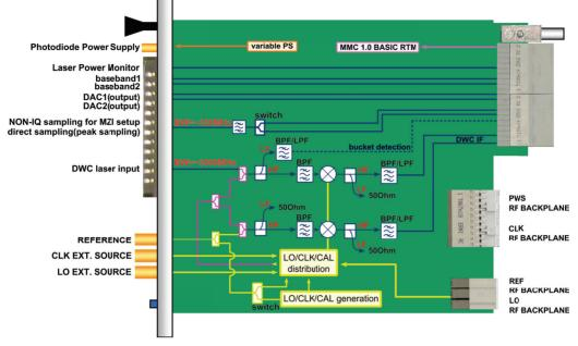
Figure 3: Block diagram of a DRTM-LASY module.
