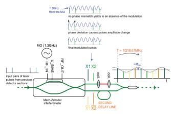
Figure 5: A scheme briefly showing phase detection in an L2RF setup. An output signal containing information about phase mismatch is in case of an MLO of frequency equal 216.67 MHz, which is also a laser pulse repetition rate. Its amplitude is proportional to the phase error.
