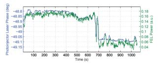
Figure 2: Observed correlation between photoinjector laser phase and FEL output power, prior to introduction of feedback.
