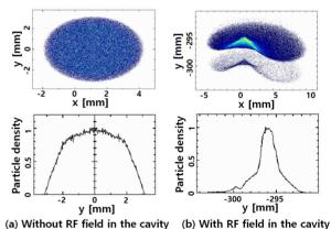
Figure 5: ASTRA simulation results. (a) is the beam distribution after the deflecting cavity without RF field in
