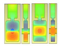
Figure 2: Electric field (left) and magnetic field (right) distribution of TM<sub>120</sub> mode in the deflecting cavity.
