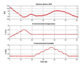
Figure 7: Libera Sync 3 long term phase drift and temperature and humidity changes.
