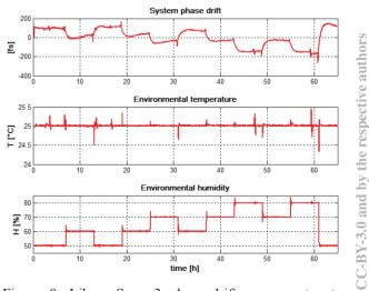
Figure 8: Libera Sync 3 phase drift response to step changes in environmental humidity.
