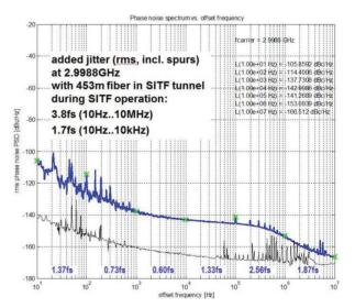
Figure 3: Libera Sync 3 added phase noise and jitter. The black curve shows the limit of the measuring setup.
