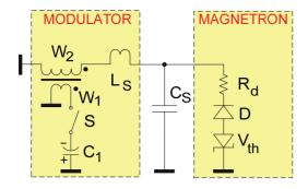
Figure 2: Modulator and magnetron equivalent circuit.
