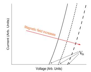
Figure 1: Volt – Ampere characteristic of a magnetron.
