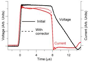
Figure 4. Current pulse shape modification.
