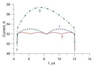
Figure 7. Current shape with different correctors.
