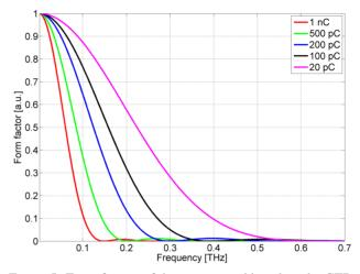
Figure 5: Form factors of the compressed bunch at the CTR station.
