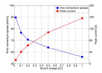
Figure 3: Simulated rms momentum spread and peak current of the compressed bunch as a function of bunch charge at the CTR station.
