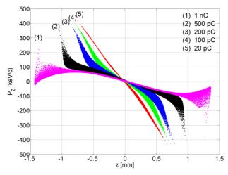
Figure 4: Simulated longitudinal phase spaces of the compressed bunch at the CTR station.
