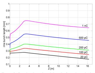
Figure 2: Simulated rms bunch lengths from the cathode (0 m) to the CTR station (16.30 m) for bunch charges of 20 pC to 1 nC.
