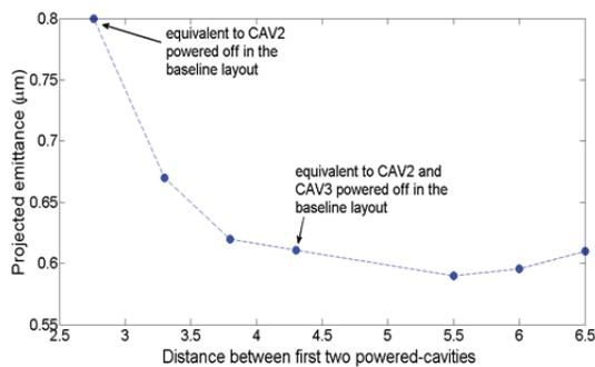
Figure 6: Emittance vs. distance between first two powered-cavities for 300 pC.
