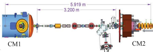
Figure 7: Schematic of the alternate layout (components from cathode to CM1 are identical to Fig. 3). Diagnostics installed in between CM1 and CM2 include the emittance station using slits, collimators, and energy spectrometer.
