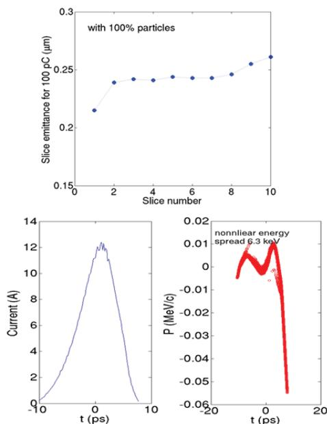
Figure 4: Slice emittance (top); longitudinal beam distribution (bottom left) and higher order energy spectrum (bottom right) at 98 MeV.
