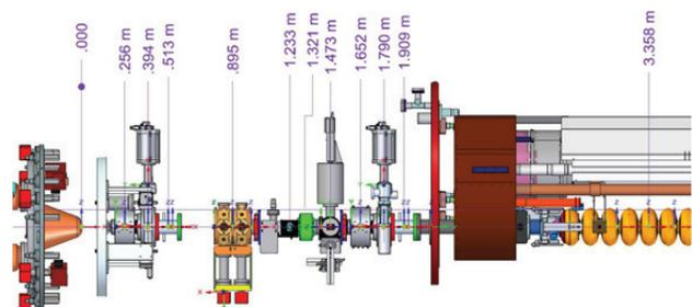
Figure 3: Schematic of new baseline layout from the cathode to CM. Major components are 186 MHz RF gun, two pairs of solenoid/BPM, 1.3 GHz NC RF buncher, ion pump, laser injection box, current diagnostic ICT, YAG screen, two valves, and standard 8-cavity CM.
