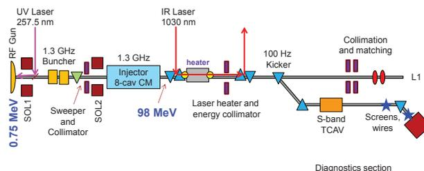
Figure 1: Schematic of the full LCLS-II injector. The front part of the injector discussed in this paper starts from the cathode to the CM end; downstream of the CM includes laser heater system, collimation systems and a dedicated beam diagnostics beamline.
