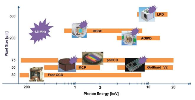
Figure 6: Planned photon detectors at the Soft and Hard X-ray beamlines. Most of them are capable of operating at the intra-bunch frequencies (4.5 MHz) [28]
