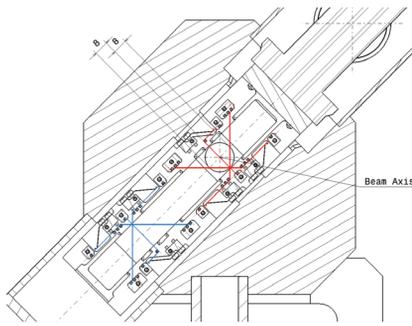
Figure 1: View of the Transverse section of the WSC vacuum chamber and, in particular, of the wire-fork and of the CF16 vacuum chamber. The wire-fork is equipped with 3 different pin-slots where the wire can be stretched. The distance of the "wire-vertex" from the vacuum-chamber axis can be set at 8, 5.5 and 3 mm in correspondence of the 3 different pin-slots.
