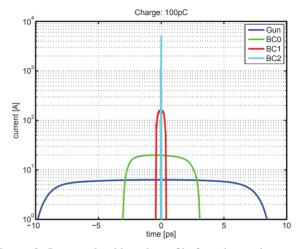
Figure 2: Longitudinal bunch profile from beam dynamics simulations.
