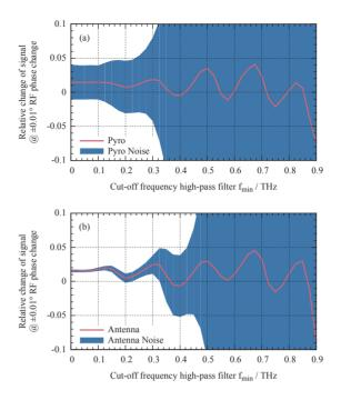
Figure 5: Simulation of relative detector response when changing RF phase by  $\pm 0.01$  deg versus edge frequency of THz high-pass filter. (a) pyro-electric sensor, (b) quasi optical detector (Schottky-diode with antenna).
