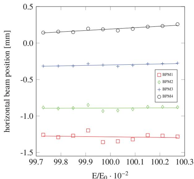
Figure 1: Results of the last dispersion measurement. This plot shows the horizontal beam positions at four different BPMs for different relative beam energies. The energy is normalized to  $E_0 = 552$  MeV.
