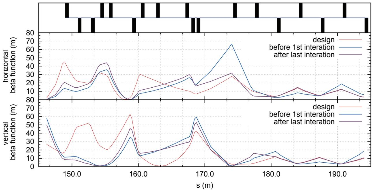
Figure 3: These plots show the design beta functions, the beta functions at the start of the matching and those at the end of this procedure. The latter match the design beta functions at the end of the seed section. The upper plot shows the horizontal plane and the lower plot the vertical plane.
