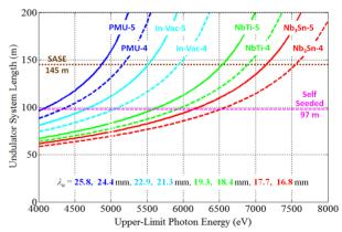
Figure 1: Undulator system length (with breaks) versus 4 upper-limit SASE photon energy saturating in 80% of that undulator length at 4 GeV. Existing 145-m und. hall length is indicated.
