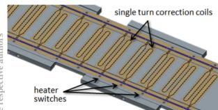
Figure 5: Periodic section field tuner on both sides of chamber.
