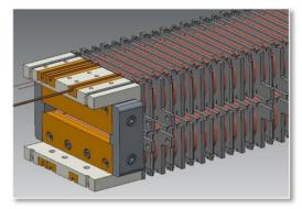
Figure 4: Nb<sub>3</sub>Sn prototype undulator magnet design.
