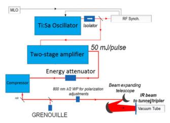
Figure 1: Schematic of the seed laser system at FLASH1.
