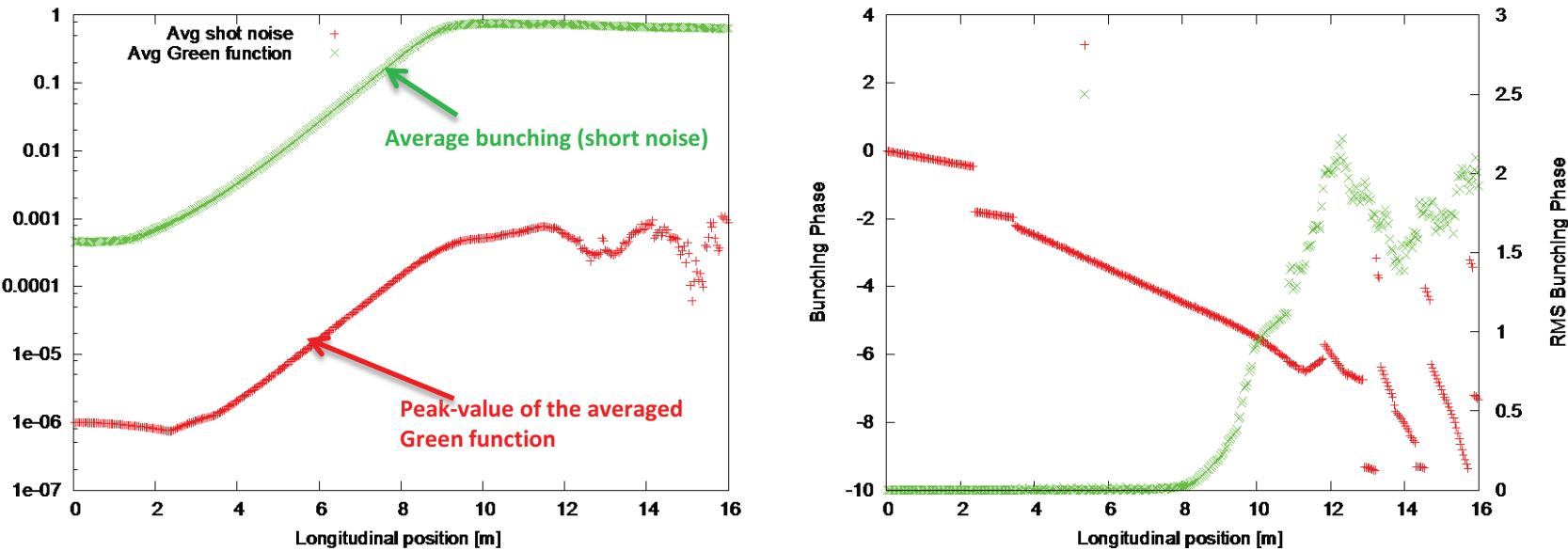
Signal grows exponentially until  $\sim 9$  m with gain at 409 and it continues to grow and saturates with gain of 777 @ 11.5 m. This is to be compared with theoretical estimation at 858.
