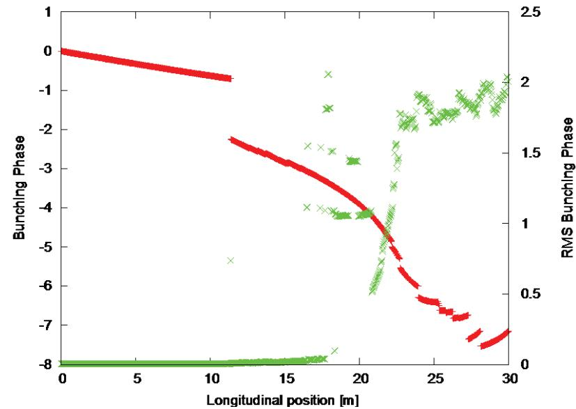
Bunching factor for the entire bunch saturates at  $\sim 20$  m ( $|b| \sim 1$ ) with noise. Signal starts to grow linearly after delay and saturates at roughly the same location as the entire bunching factor. Max gain of bunching factor at 20 m is 27 and the theoretical estimation gives 29.4.
