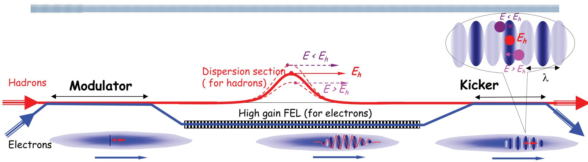
FEL amplifies the initial energy variation proton beam imprints on the electron beam and the amplified signal is used as a FB to correct proton beam downstream.
