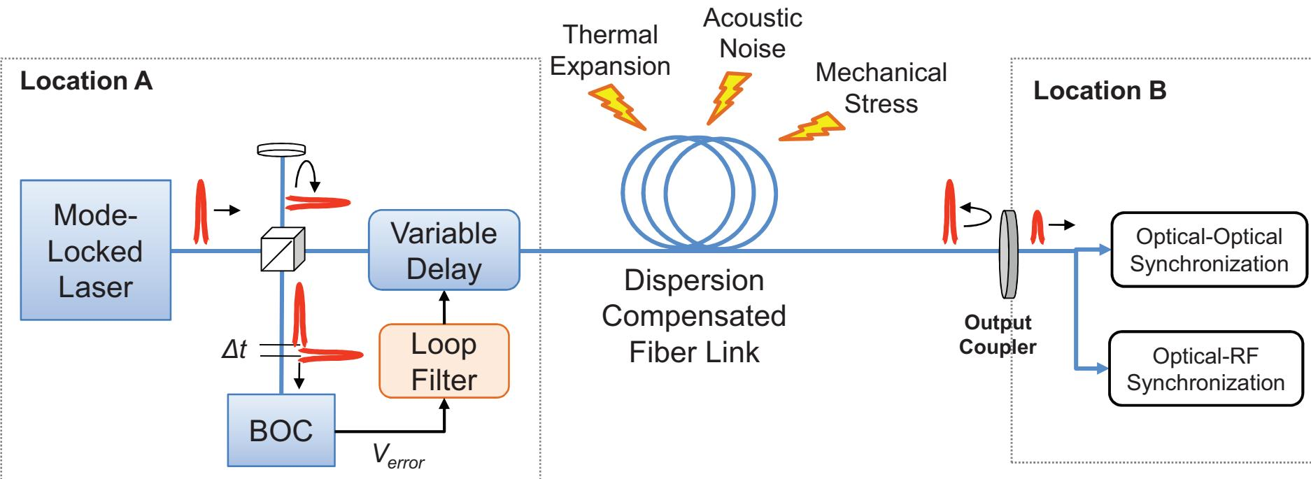
1. Detect timing error at link input
