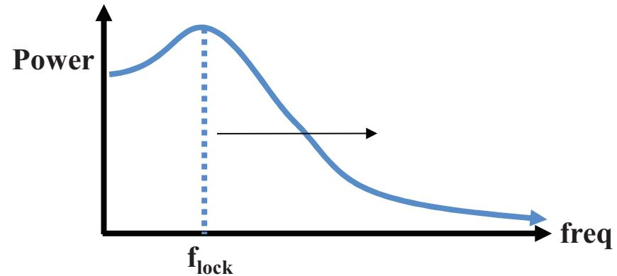
✓ Timing jitter outside the locking bandwidth measured by SSA
