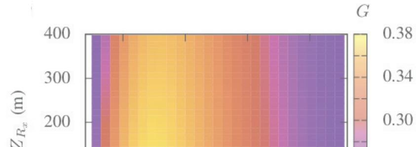
Simulated image of the mode shape at the undulator center, showing a mode size aspect ratio of about 3.7 : 1 (compare to e-beam elongation 20 : 1)
