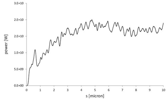
Figure 8: Power distribution along the last (6) bunch.
