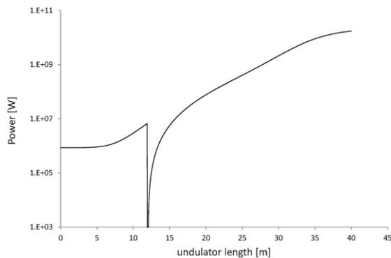
Figure 7: Power gain in X-ray cavity and output undulators.
