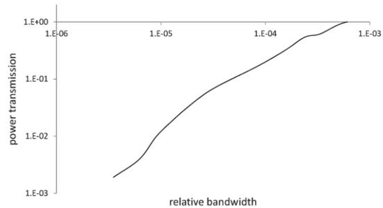
Figure 5: Power transmission as a function of the reflection filtering.
