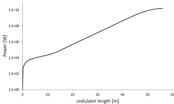
Figure 2: Power gain along undulators.
