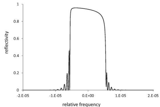
Figure 6: Spectrum reflectivity of four diamond (311) crystals.
