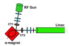
Figure 3: Layout of the injector section of the linac-based THz source facility at Chiang Mai University.
