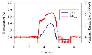
Figure 8: Measured electron macro-pulse downstream the RF-gun  $(I_{CT1})$  and the simulated maximum kinetic energy along the macro-pulse.
