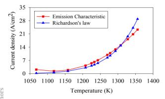
Figure 2: Emission current densities of the thermionic cathode as a function of the cathode temperature.
