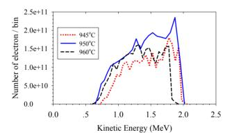
Figure 5: Energy spectrum of electron beam measured at the CT2 for the cathode temperature of 945°C, 950°C and 960°C.
