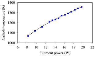
Figure 1: Relationship between the cathode filament power and the measured cathode temperature.
