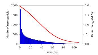
Figure 9: Particle distribution and histogram in energytime phase space for a simulated single bunch at the RFgun exit for the maximum beam kinetic energy of 2 MeV.
