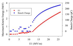
Figure 7: Simulated maximum kinetic energy ( $KE_{max}$ ) and emitted bunch charge of electron as a function of the average accelerating field at the cathode ( $E_1$ ).
