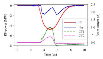
Figure 4: Waveforms of the forward ( $P_f$ ), reflected ( $P_{re}$ ) RF pulses and the typical electron macro-pulses downstream the RF-gun ( $I_{CT1}$ ) and downstream the alpha magnet ( $I_{CT2}$ ).
