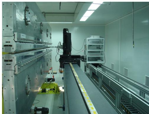
Figure 1 : The undulator measurement bench with U48 of EXFEL under test
