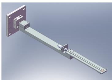
Figure 4: The structure of the magnetic sensors holder
