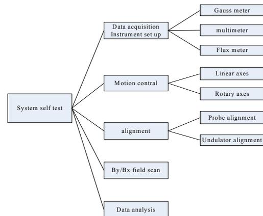
Figure 2: Measurement program block diagram
