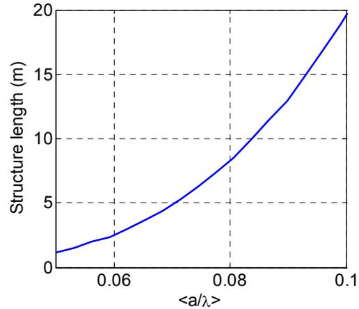
Figure 1: Constant-gradient structure length as a function of average iris radius, normalized to the rf wavelength.
