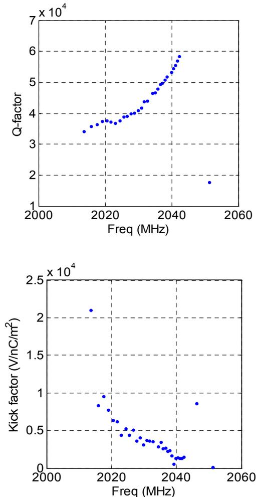
Figure 2: The Q-factors (top) and transverse kick factors (bottom) for the first dipole passband of the structure.
