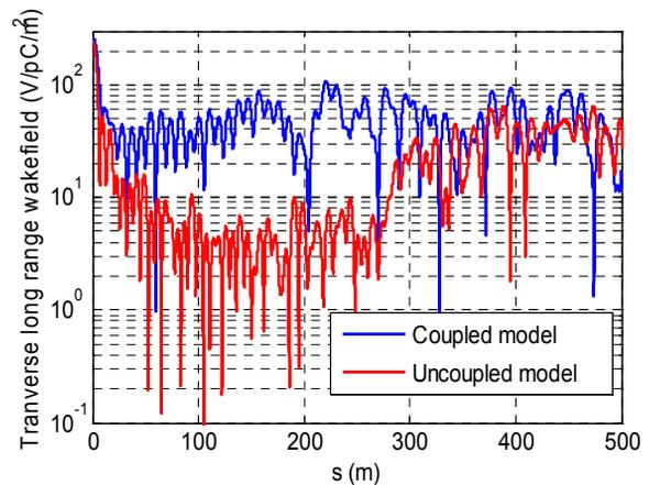
Figure 3: Transverse wakefield envelope as a function of the distance,  $s$ , behind the bunch.
