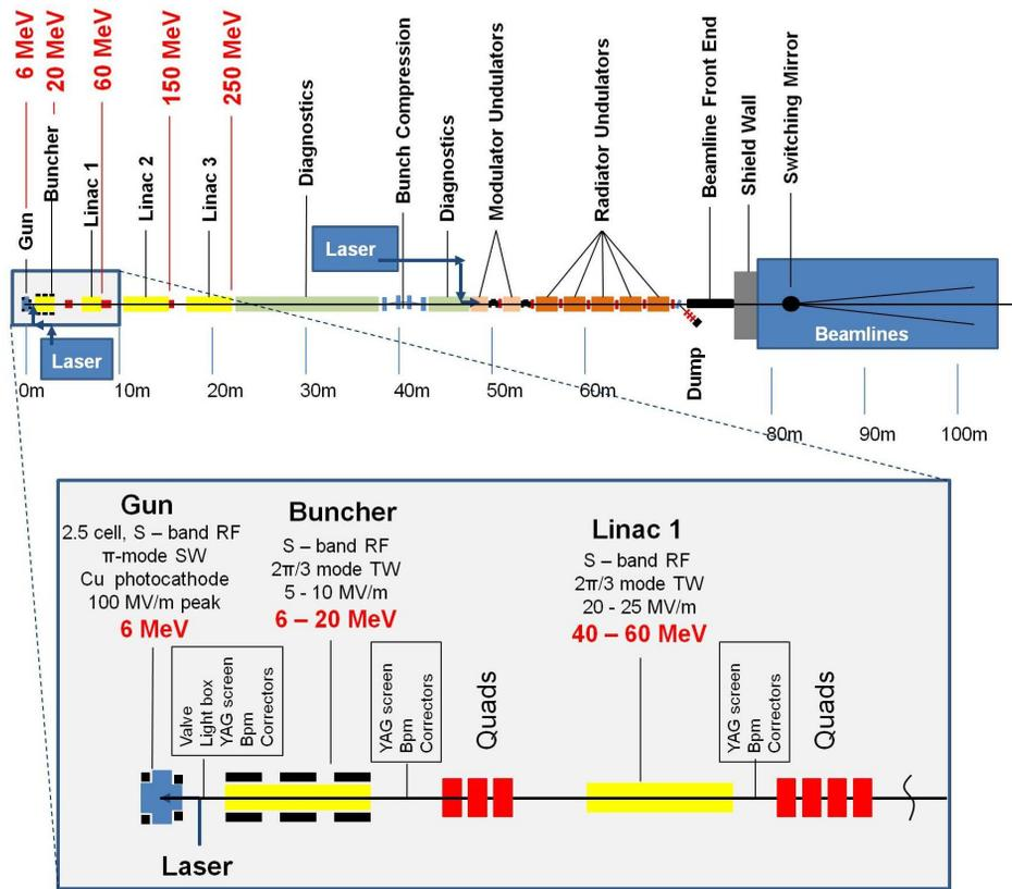
Figure 1: Provisional CLARA Layout (top) and enlarged view of first 10 m (bottom).
