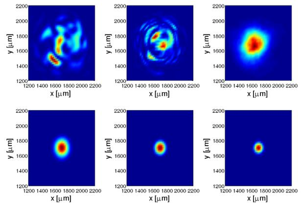
Figure 4: FEL amplification output at different positions, SASE mode (upper) vs. HGHG (lower).
