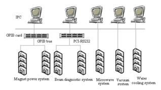
Figure 1: Architecture of the FEL control system
