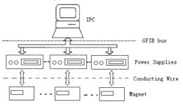
Figure 2: Architecture of the power supply system
