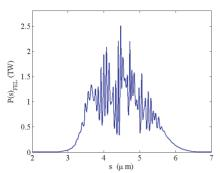
Figure 3: The instantaneous, 8.3-keV power profile at  $z=160\,\mathrm{m}$  in the second undulator according to time-dependent GENESIS simulation.
