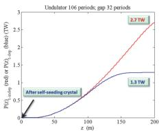
Figure 1: GENESIS predictions for amplification of a 5-MW seed in a tapered, 200-m long undulator for time-steady (red), full time-dependent "fresh" bunch (blue), and start-to-end (green) conditions.
