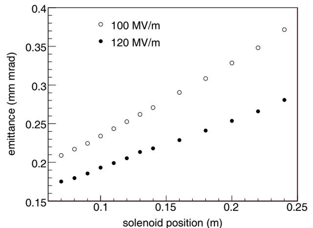
Figure 4: Normalized transverse emittance as a function of the distance between the solenoid center and the cathode at 100 and 120 MV/m peak RF field at the cathode. The simulations were carried out at 200 pC bunch charge.
