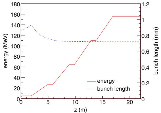
Figure 6: Beam energy and bunch length evolution at 200 pC bunch charge and 120 MV/m gun peak field. The bunch length becomes shorter as the beam propagates through the first accelerating section. The RF phase of the first section was  $-60^\circ$  from the on-crest phase.
