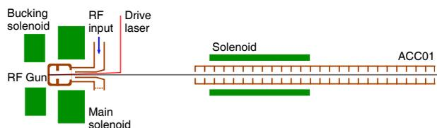
Figure 1: Layout of the first part of the photoinjector. Three more accelerating sections (not shown) follow ACC01 for accelerating a beam to a space charge free regime.
