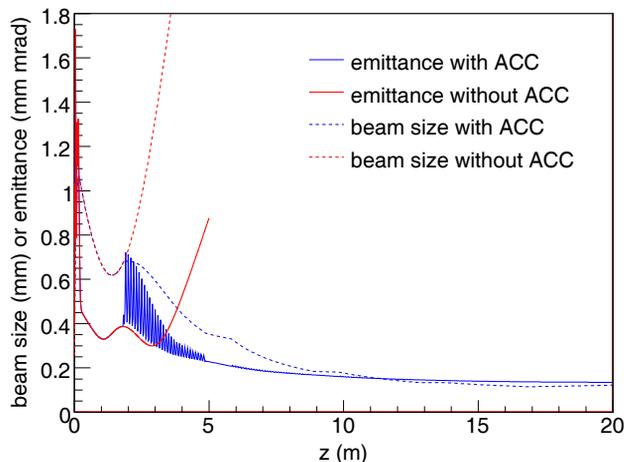
Figure 5: Beam size and emittance evolution from the cathode to the injector end, with and without accelerating sections. 200 pC bunch charge and 120 MV/m peak gun field were used for ASTRA simulation.
