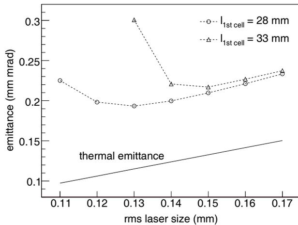
Figure 3: Normalized transverse emittance at the gun exit for various laser sizes. The two first cell lengths ( $l_{1st\ cell}$ ), 28 and 33 mm, were studied. The thermal emittance is shown for comparison. The same simulation conditions were used as in Fig. 2 unless otherwise mentioned.
