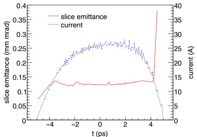
Figure 7: Slice emittance and current profile of a 200 pC beam at the end of the injector.
