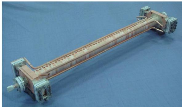
Figure 1: 1<sup>st</sup> prototype C-band accelerating structure.
