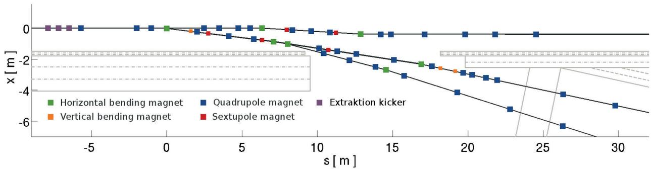
Figure 1: This plot shows a top view of the arc including FLASH on top and of the new beamline of FLASH2 in the middle. The lowest beamline shows a first design of FLASH3. The building walls are sketched in Grey color.
