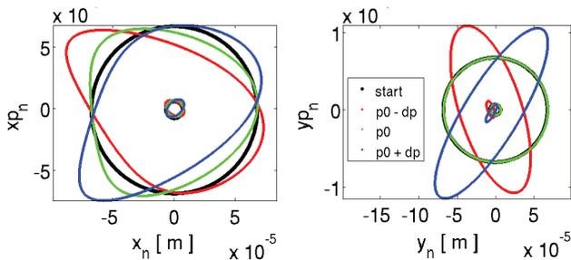
Figure 3: 3- $\sigma$ -ellipses with  $\pm 0.5\%$  energy deviation in normalized horizontal and normalized vertical phase space.
