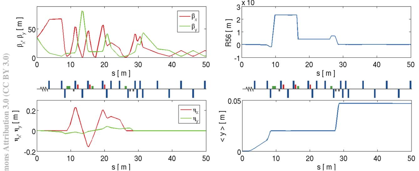
Figure 2: Optic functions for the FLASH2 extraction arc. The upper plots show the betatron functions and the first order momentum compaction (R56) and the lower the dispersion and the vertical beam center position.
