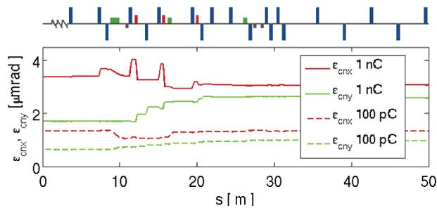
Figure 5: S2E simulations with two typical particle distributions with 100 pC and 1 nC charge.
