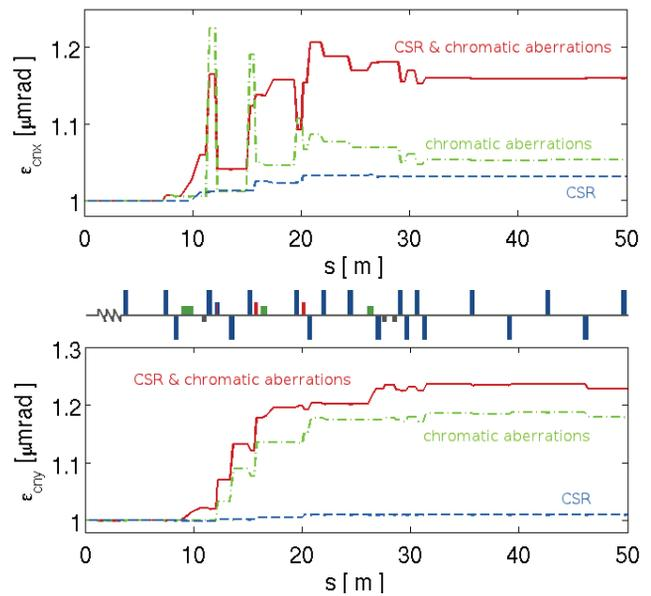
Figure 4: Plots of the results to compare the impact of CSR and chromatic aberration on the projected emittance.
