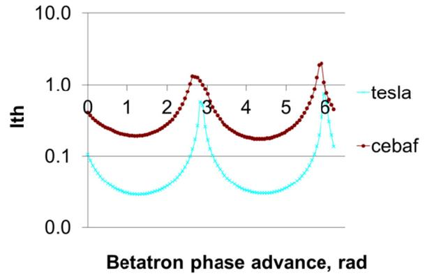
Figure 2: Comparison of the threshold currents for TESLA and CEBAF type linacs for BERLinPro.
