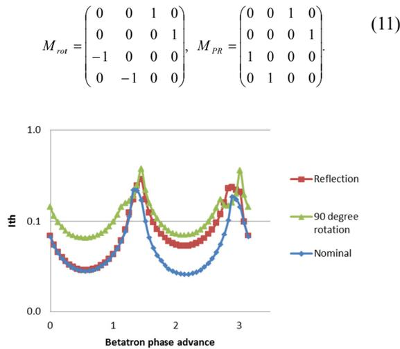
Figure 5: The results of BBU modelling for BERLinPro with rotator and solenoid.
