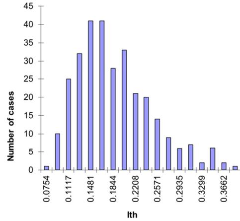
Figure 3: Results of BBU modelling for TESLA type linac. The optics was chosen correspondingly to the maximum current value from Fig. 2.  $\sigma = 1$  MHz..
