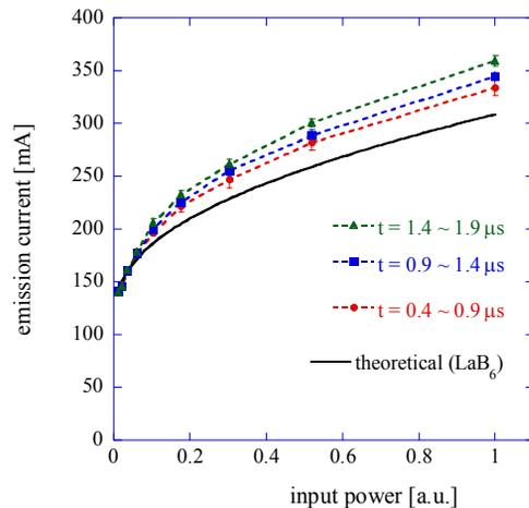
Figure 7: Power dependence of emission current. Solid line shows the expectation given by eq. (1).
