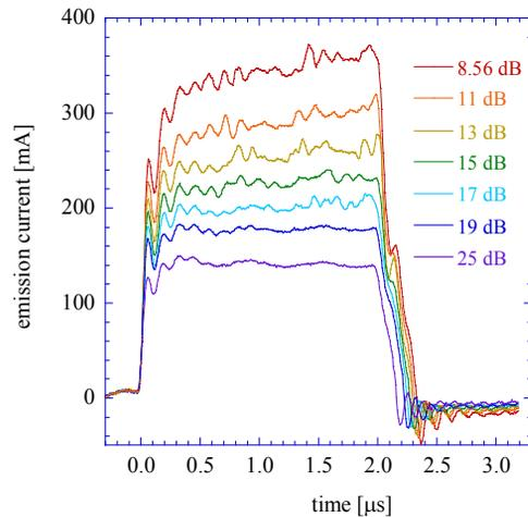
Figure 6: Observed CT signal placed in the heater line for the several input power levels. Heater current = 9 A. Each waveform is averaged over 16 times.
