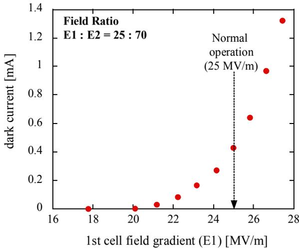
Figure 5: Measured dark current. The field gradient in the first cell was varied keeping the field ratio to 70/25 for the second cell.
