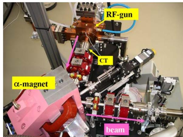
Figure 2: Injector part of t-ACTS. Extracted beam from the gun is measured by the current monitor (CT).
