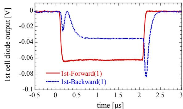
Figure 4: Measured waveform of input and reflection power for the first cell.
