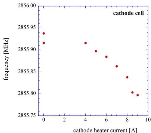
Figure 3: Frequency shift due to the cathode heater power.
