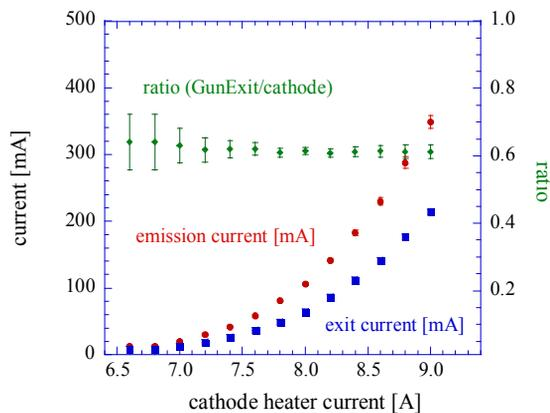
Figure 8: Heater current dependence of emission current.
