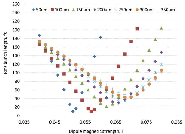
Figure 3: Rms bunch length after the chicane for different magnetic strengths inside the dipoles (Gaussian temporal laser profile).
