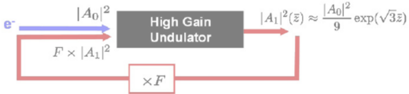
Fig. 1. Schematic representation of a generic high gain RAFEL system.
