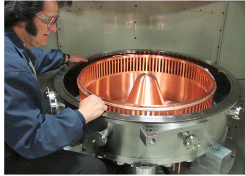
Figure 2: The VHF cavity during the final phase of the fabrication.
