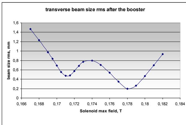
Figure 3: Transverse beam size rms at the end of the booster for the solenoid scan at 500pC
