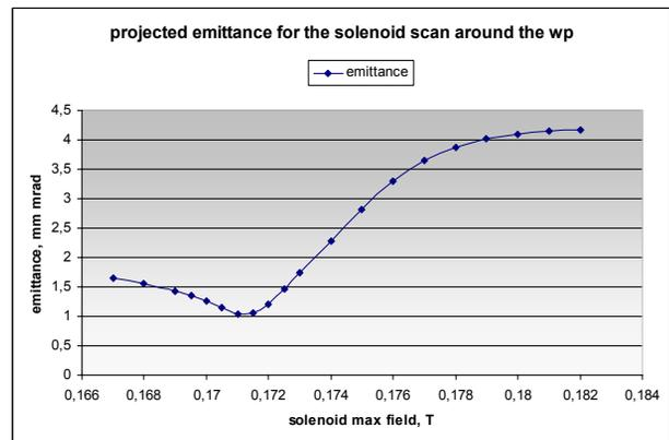
Figure 1: Projected emittance for the solenoid scan round the working point for 500 pC
