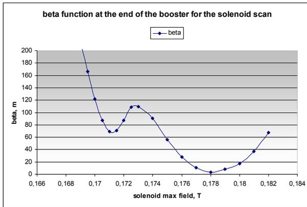
Figure 2: Beta function at the end of the booster for the solenoid scan at 500pC. The optimal value for the solenoid field with respect to the emittance was found to be 0.1715T. At this point the beta function has a local minimum though, but it achieves its absolute minimum for the field strength of 0.1718T.
