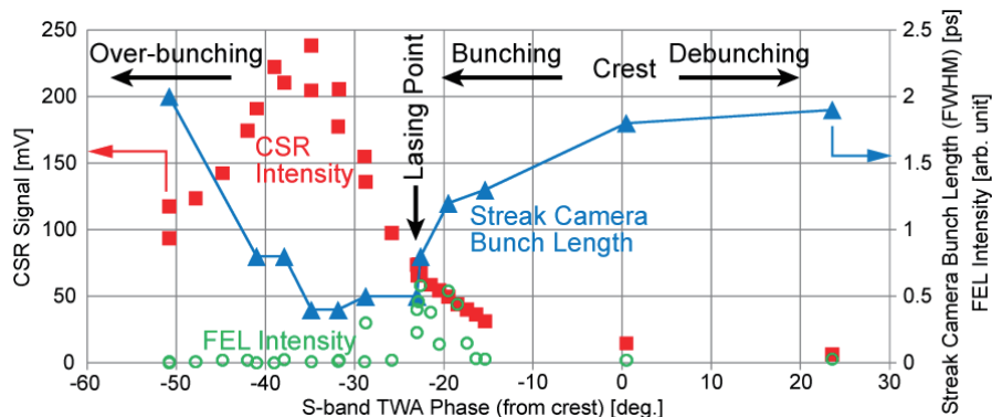
Figure 7: The CSR intensity detected by the pyro-electric detector (red square) and the bunch length measured by the streak camera (blue triangle). The horizontal axis is the rf phase of the S-band TWA. The origin of the horizontal axis is the crest acceleration phase. The FEL intensity is also plotted (green circle).
