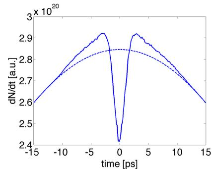
Figure 1: Charge distribution of the sliced electron bunch at the SLS right after the slicing.
