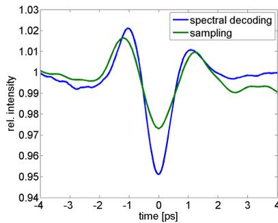
Figure 6: Arrival time jitter corrected average of 500 EOSD measurements of turn 0 and the corresponding sampling measurement
