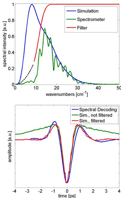
Figure 7: top: measured spectrum of the sliced bunch at turn 0 highpass filter (green), the spectrum derived from particle tracking simulations (blue), and the assumed transfer function of the IR beamline, bottom: EOSD measurement (blue) compared to the simulation directly (green) and the simulation filtered with the assumed transfer function of the IR beamline (red).
