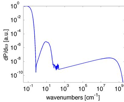
Figure 2: Spectrum of the synchrotron radiation emitted from the sliced electron bunch
