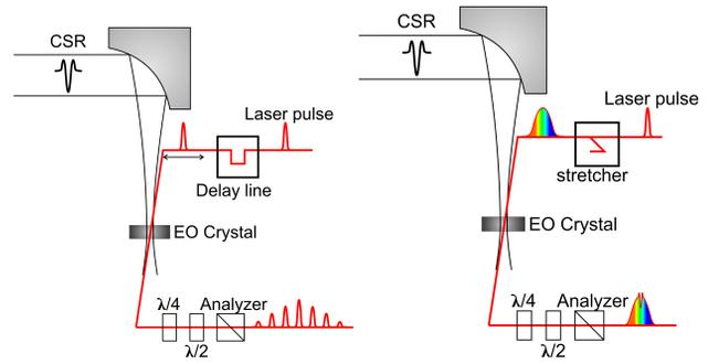
Figure 3: Scheme of the setup for EO sampling (EOS, left) and spectrally decoded detection (EOSD, right)
