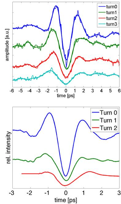
Figure 4: EO sampling measurements of turn 0 to 3 and EO spectral decoding measurements of turn 0 to 2
