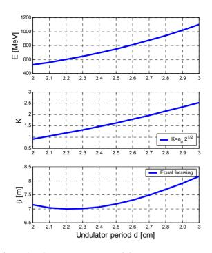
Figure 2: Electron energy *E*, undulator parameter *K* and equal-focusing  $\beta$ -function as functions of the undulator period *d*. H<sub>C</sub>=13kOe, the undulator gap *g*=1 cm.
