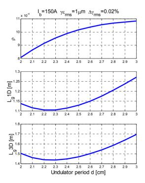
Figure 3: The Pierce parameter  $\rho$ , one-dimensional gain length L<sub>g</sub>1D and actual gain length L<sub>g</sub>3D as functions of the undulator period *d*. L<sub>g</sub>3D was calculated according to parametric formula [12].
