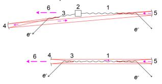
Figure 4: Two schemes of the regenerative amplifier FEL exploiting electron outcoupling technique. Top: with ebeam bending. Bottom: with tapering. 1 - main undulator, 2 - achromatic bend, 3 - last undulator section, 4 and 5 - mirrors, 6 - radiation from the main undulator. Radiation used for feedback is shown by red lines and small violet arrows.
