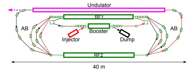
Figure 1: The scheme of ERL with FEL. RF1 and RF2 – RF accelerating structures, AB – achromatic bends. Red arrows – accelerating "fresh" beam, black arrows – decelerating used beam.
