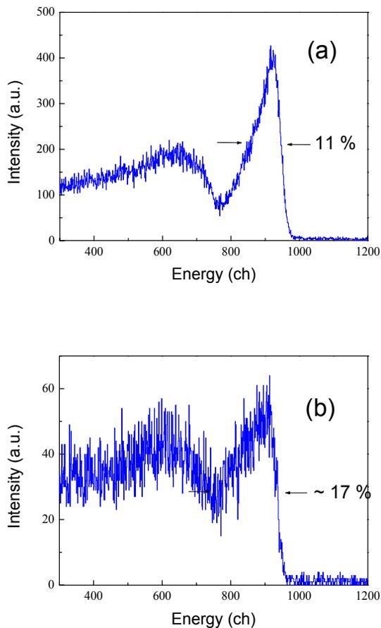
Figure 4: Energy spectra of the inverse Compton X-rays scattered from the points outside the undulator (A) and inside the undulator (B). 950 ch in the transverse axis corresponds to the photon energy of 1.2 MeV.
