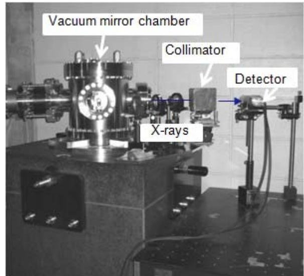
Figure 2: Setup of the X-ray detection system.
