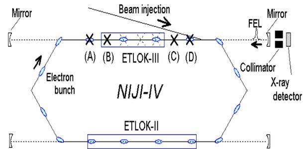
Figure 3: Schematic drawing of Compton collisions in the NIJI-IV FEL system.
