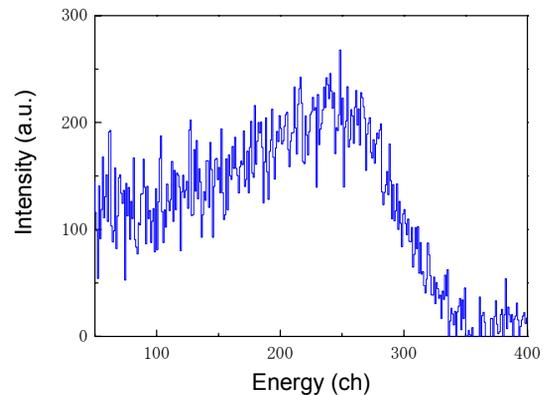
Figure 5: Typical X-ray spectrum in the random collision mode. 350 ch in the transverse axis corresponds to the photon energy of 6.1 MeV.
