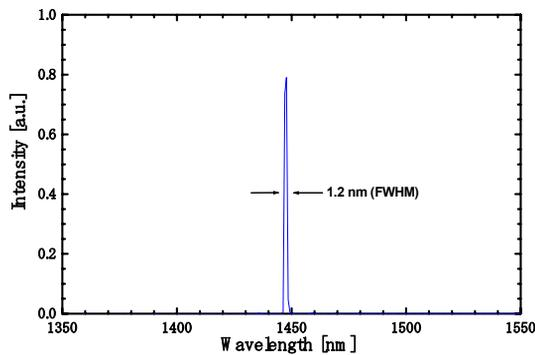
Figure 1: Typical FEL spectrum around 1.45  $\mu\text{m}$ .
