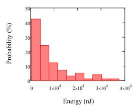
Figure 18: Histogram of the pulse energy obtained with the untapered undulator.
