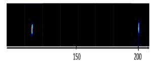
Figure 6: Spectral range from 115 up to 205.85 nm is shown with the presence of the second and the third harmonics (132.66 nm and 199 nm).
