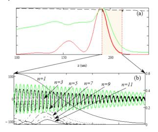
Figure 7: Graphical representation of the radiation pulse slipping from left to right in the e-beam frame (red) and of the induced energy spread (green) (Fig.7a). Longitudinal e-beam phase space in the front part of the pulse (Fig.7b). In Fig.7b the square moduli of the bunching coefficients for the first eleven (odd) harmonics are plotted. The green line represents the motion separatrix whose envelope is proportional to the square root of the laser field (simulation with PERSEO TD).
