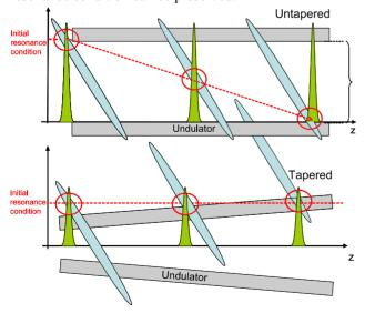
Figure 13: The pictures represent the propagation of a field spike (green) developing on the rear part of a chirped e-beam (light blue). The upper diagram is
