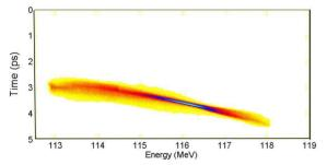
Figure 14: Longitudinal phase space reconstruction at the exit of the linear accelerator.
