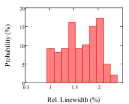
Figure 17: Histogram of the spectral width obtained with the untapered undulator, with the resonance set at 540nm.
