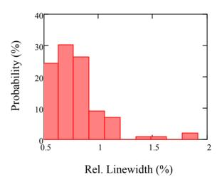
Figure 21: Histogram of the relative linewidth obtained with the tapered undulator.
