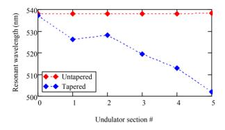
Figure 19: Resonant frequency in the six undulators in the untapered and tapered case.
