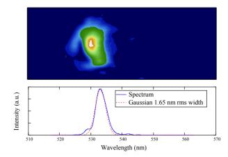
Figure 22: Typical spectrum showing a single coherence region (single spike).
