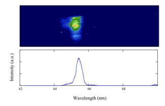
Figure 11: Spectrum of the third harmonic of the radiator.
