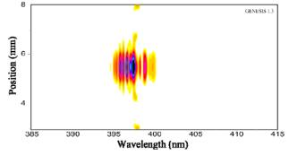
Figure 3: GENESIS 1.3 data, obtained with the following data: I=65A,  $\varepsilon_x$ =2.9 mm mrad,  $\varepsilon_v$ =2.5 mm mrad (norm.).
