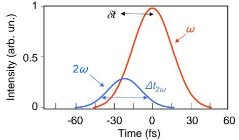
Simple system but only relative control on the 2<sup>nd</sup> harmonic generation parameters (mainly the BBO thickness):
